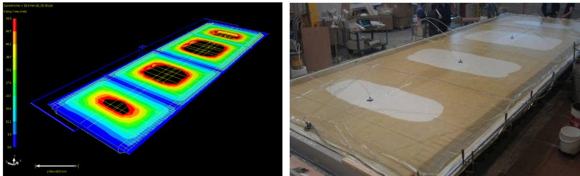
Figure 7 Flow-simulation (left) and vacuum-infusion of the panels in production (right).
