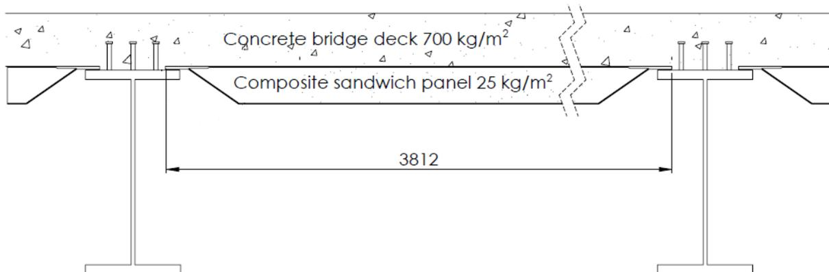
*Figure 2 Principle of composite sandwichpanel as formwork for casting concrete.*
