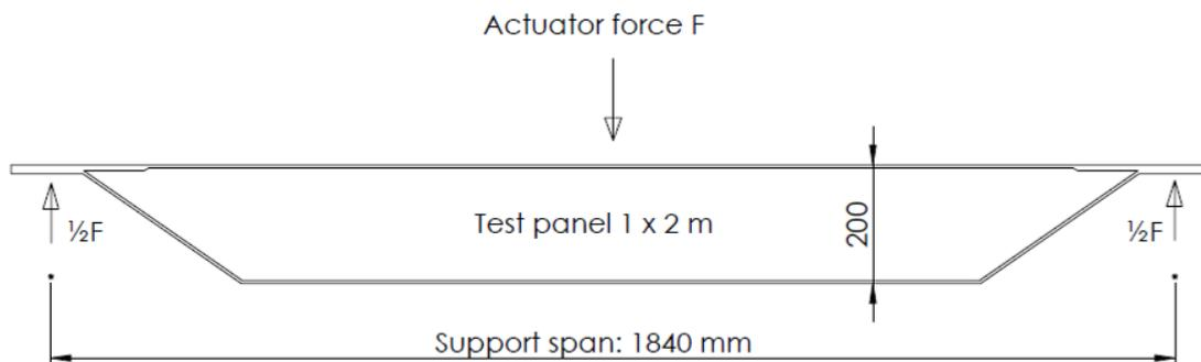
Figure 5 Set-up for three-point bending test on test-panels.
