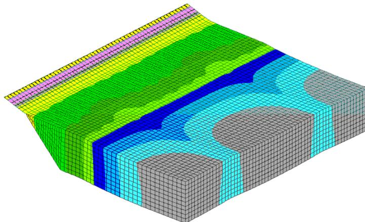
Figure 4 Contour plot of vertical displacement of the FEM-model.
