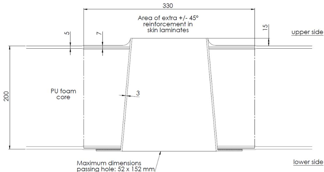
Figure 6 Cross-section and dimensions of a passing hole.
