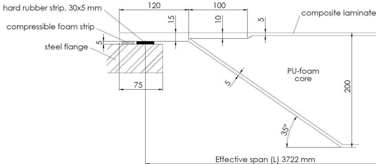
Figure 3 Details of supporting edge of the composite panel.
